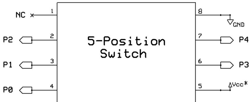
\*Vcc = 3.3V for Propeller Applications
