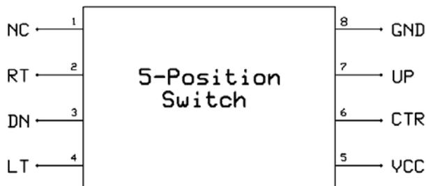
\*Supply voltage will determine output voltage. Be sure to use a supply voltage that your microcontroller will tolerate as an input signal.
